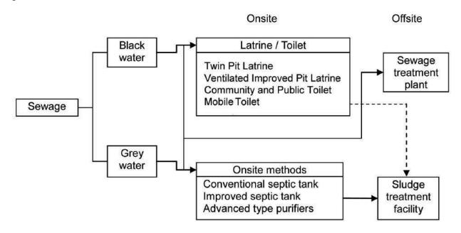
Figure 8.3 On-site and Off-site sewage treatment system
