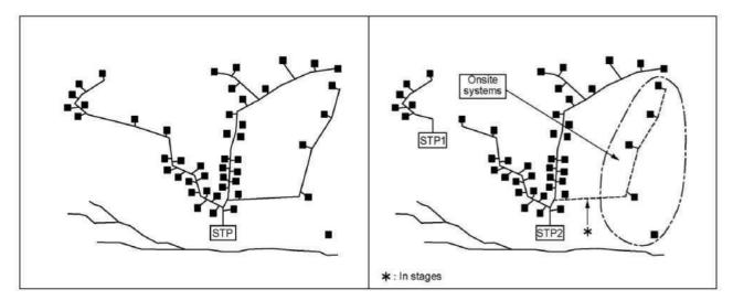
Figure 8.2 Concept of centralized system at left Vs. decentralized system at right
