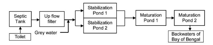
Figure 8.9 Schematic of the twin drain decentralized sewerage
