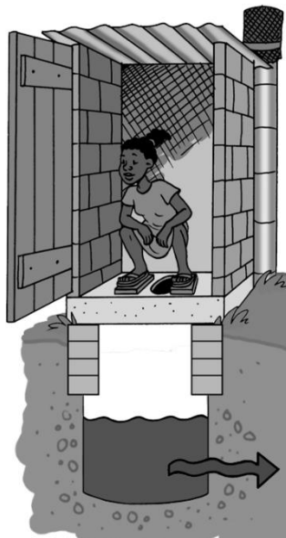
Fecal sludge collected in a pit latrine
