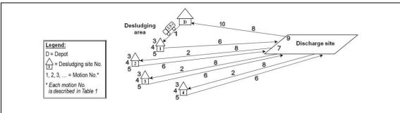
Figure 1. Overview of desludging cycles in one day (4 cycles in the present case)
