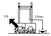
Figure 5.4. Double vault no-mix latrine (FS = faecal solids)
