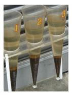
Conducting a Jar Test for Evaluating Sand Drying Bed Media
