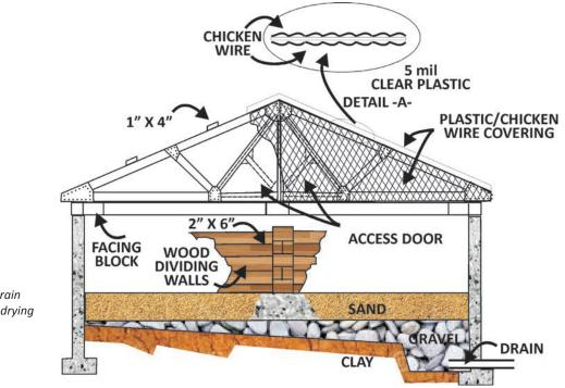
Figure 9. Underdrain system of a sand-drying bed.
