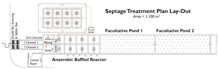
Figure 19. Initial site plan drawing for a hypothetical septage treatment facility.
