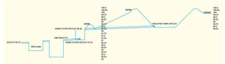
Figure 4. Hydraulic gradient using gravity flow.
