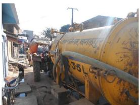
Figure 2: Desludging Vehicle
