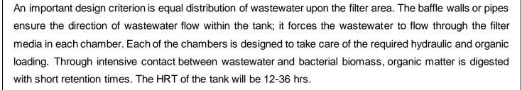
Anaerobic filters are suitable for domestic wastewater with low content of suspended solids. In any case pretreatment is necessary to prevent clogging. Suspended solids and BOD removal of 85-90% can be achieved.
