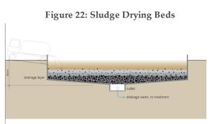
of the pipes are layers of gravel and sand that support the sludge and allow the liquid to infiltrate and collect in the pipe. While the solid fraction remains on the filter surface and is dried by natural evaporation, the liquid percolates. Sludge is applied in layers on top of the gravel beds and is naturally dried. It should not be applied in layers that are too thick as this will deter drying. The final moisture content after 10 to 15 days of drying should be approximately 60%.
