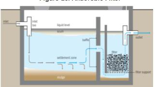
Figure 26: Anaerobic Filter
