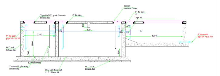
Figure 14: Cross Section of Stabilisation Reactor
