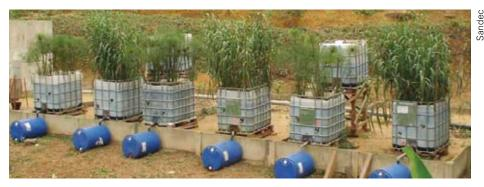
Photo 1: Pilot beds of the VFCW developed for the FS dewatering study in sub-Saharan countries.
