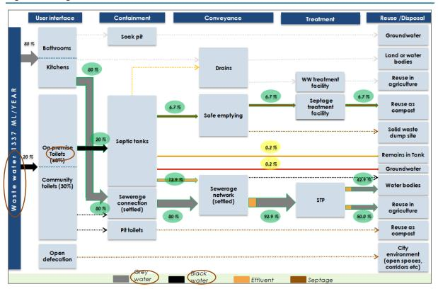
Figure 22: Targetted wastewater flow after CSP interventions
