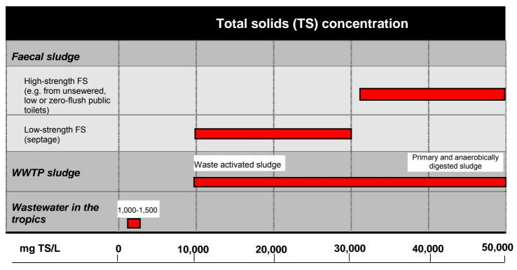
Fig. 6 Solids contents of faecal sludges, WWTP sludges and tropical wastewater
