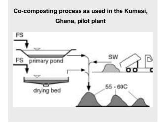
**Fig. 17** Co-Composting Flow Chart – the faecal sludge needs to be dewatered or thickened to enable the treatment of inhabitant-equivalent quantities of FS and solid waste
