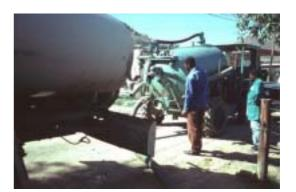
Photo 4 Transboarding of FS from a Mini-Tanker to A Standard-Size Vacuum Tanker (Maseru, Lesotho)
