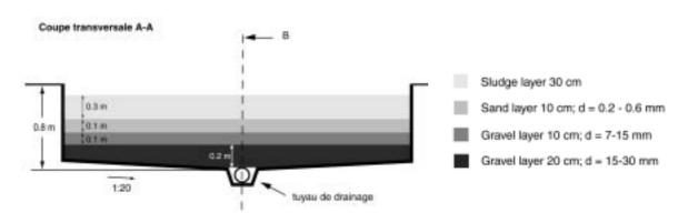
Fig. 10 Unplanted sludge drying beds (schematic)
