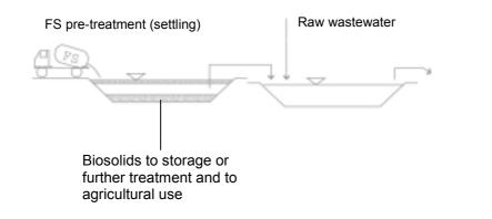
**Fig. 14** Co-treatment of FS and wastewater in ponds (schematic)
