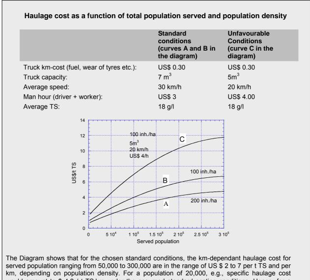
would amount to \$ 4.2 / t TS·km under the assumed standard costing conditions. Hence, for a treatment plant located 10 km outside the settlement area, the haulage cost would amount to \$ 42 / t TS·km. Under unfavourable conditions (unpaved roads, higher salaries and smaller trucks), haulage cost per km as per this model may be as high as \$ 10.5 per t TS.
